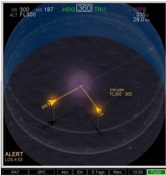
**Figure 1.** Cockpit display of traffic information. Image shows Toggle condition View 1, conflict with an intruder in a crossing conflict from the left and traveling at the same speed and same altitude as Ownship.
