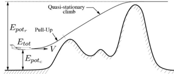
**Figure 4** How fast an aircraft is able to exchange its kinetic energy into the potential energy level that is required ( $E_{pot,r}$ ) to safely pass over the terrain is limited by the pull-up maneuver and climb performance.
