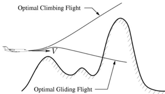
**Figure 5** The performance limitations can be used to detect a possible threat to safety. Here, the aircraft can still fly over the mountain ridge when initiating the optimal climb. However, in case of total engine failure an evasive maneuver in the horizontal plane will be required.
