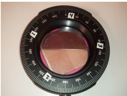
FIG. 5. Fabricated wire grid polarizer mounted in an optical rotation stage.
