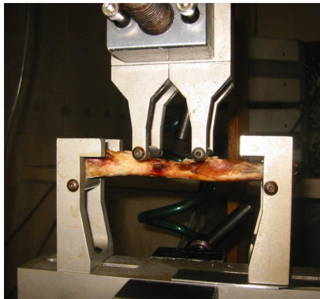
Fig. 1. Intact clavicle placed in four point bending apparatus.
