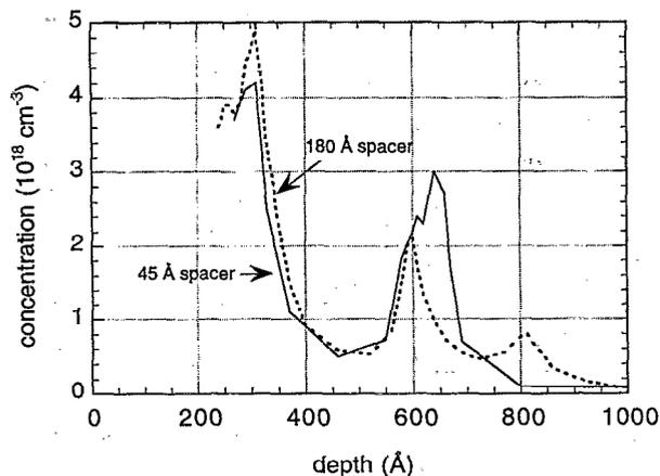
FIG. 2. Electrochemical  $C$ - $V$  profiles of  $p$ HEMT samples with different spacer layer thicknesses: (—), 45 Å spacer; (---), 180 Å spacer. Details of the structure are given in Fig. 1.
