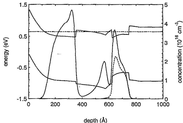
FIG. 3. Self-consistent  $\mathbf{k} \cdot \mathbf{p}$  calculation of the bands and electron concentration of a  $p$ HEMT sample with a 350 Å cap and a 45 Å spacer layer. Details of the structure are given in Fig. 1. Also shown is the electron concentration only (---) of the same structure except with the cap removed. Note that, in the latter case, the  $\delta$  region is almost completely devoid of electrons, and the well region much reduced. The chained line is the Fermi level.
