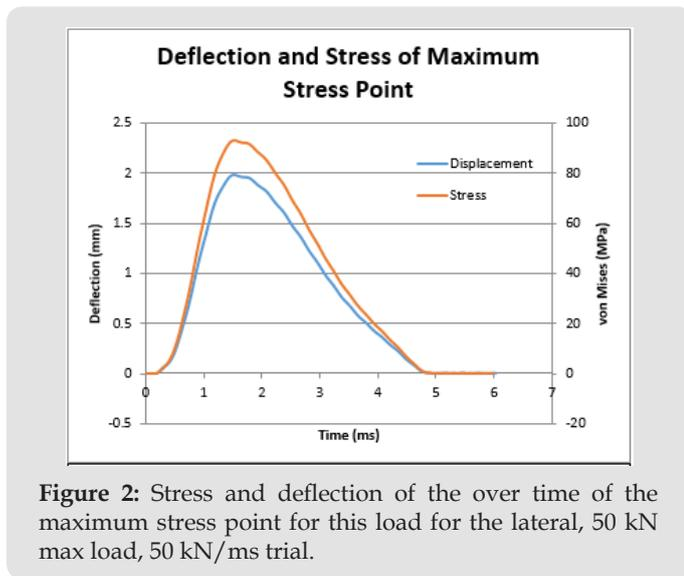
**Figure 2:** Stress and deflection of the over time of the maximum stress point for this load for the lateral, 50 kN max load, 50 kN/ms trial.
