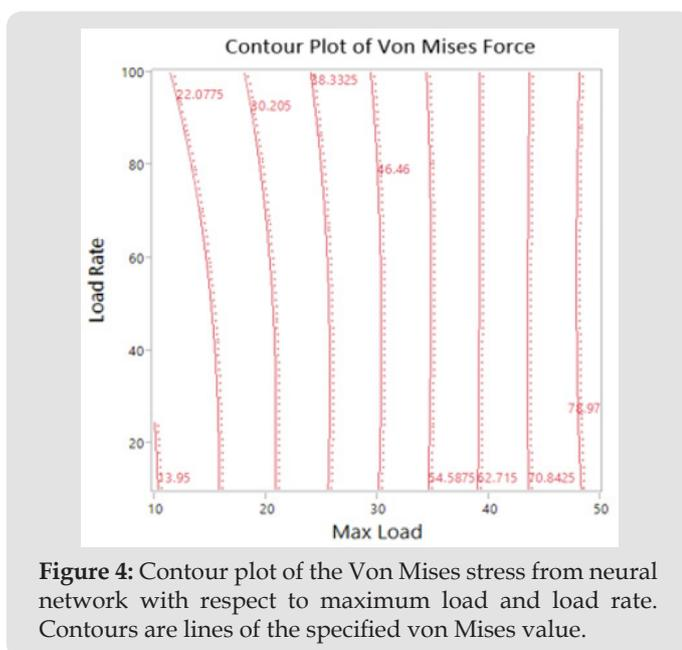
**Figure 4:** Contour plot of the Von Mises stress from neural network with respect to maximum load and load rate. Contours are lines of the specified von Mises value.
