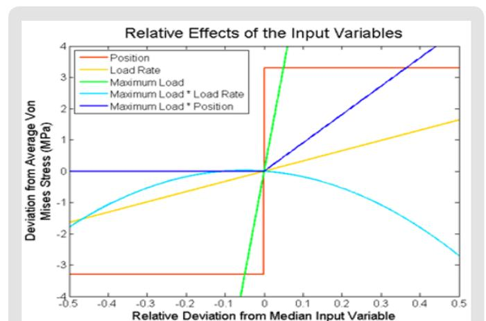
**Figure 3:** Relative scale of the effects of the input variables on von Mises stress based on least squares analysis. All variables were scaled from their minimum and maximum inputs to fit from -0.5 to 0.5. For example, -0.5 corresponds to the minimum load rate of 10 kN/ms, while 0.5 corresponds to a load rate of 100 kN/ms.
