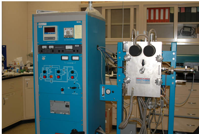
Fig. 16. A picture of the graphite resistance furnace used at Wright-Patterson Air Force Base to grow the carbon nanotubes.
