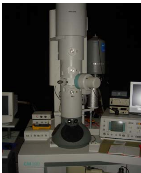
Fig. 24. Philips CM-200 field emission gun (FEG) TEM operated at 200 kV.
