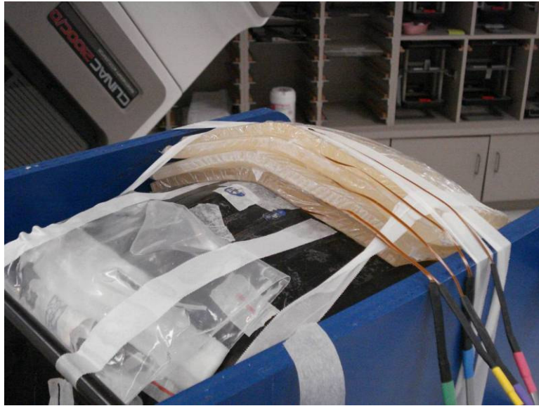
Figure 3.6: Rando with MOSFETs and Fabricated Breast Material
