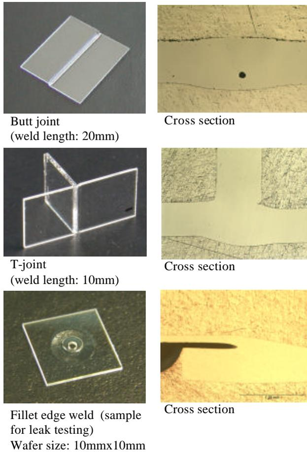
Figure 1: Laser welded glass samples (material: Pyrex 7740)
