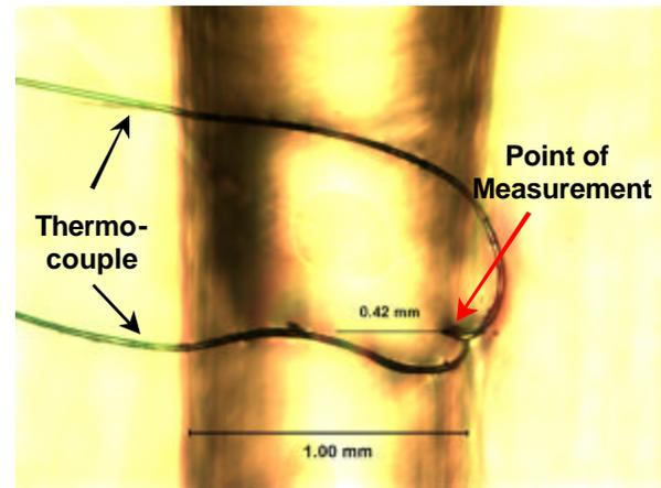
Figure 2: Penetration overlap weld with thermocouple
