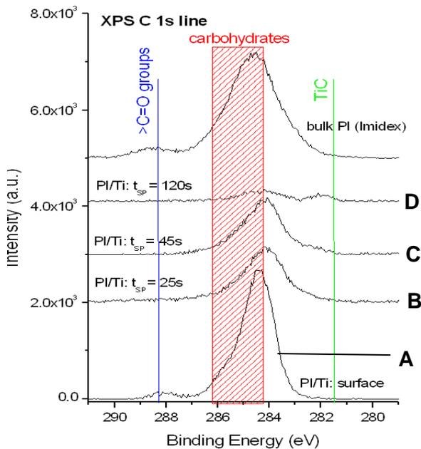
Figure 7: XPS spectra of the polyimide-titanium bond interface
