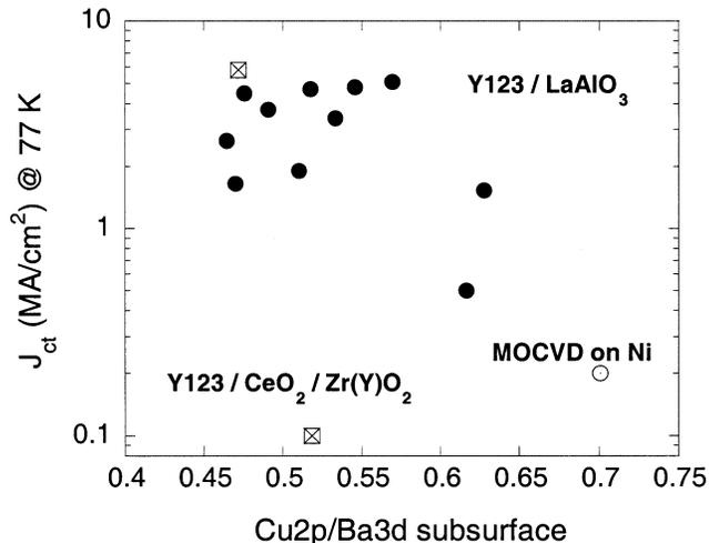
Fig. 4. Correlation of the peak intensity ratios for the  $Cu(2p)/Ba(3d)$  peaks as determined by XPS and the critical transport current as determined by the four probe resistive technique. The sample preparation methods are labeled in the figure.
