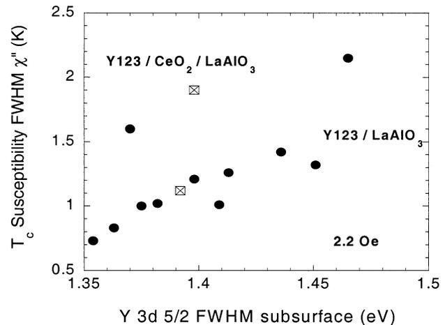
Fig. 2. Correlation of the FWHM for the  $\text{Y}(3d_{5/2})$  peak as determined by XPS and the FWHM of the critical transition temperature as determined by magnetic susceptibility measurements. The sample preparation methods are labeled in the figure.  $T_c$  data determined in 2.2 Oe magnetic field.
