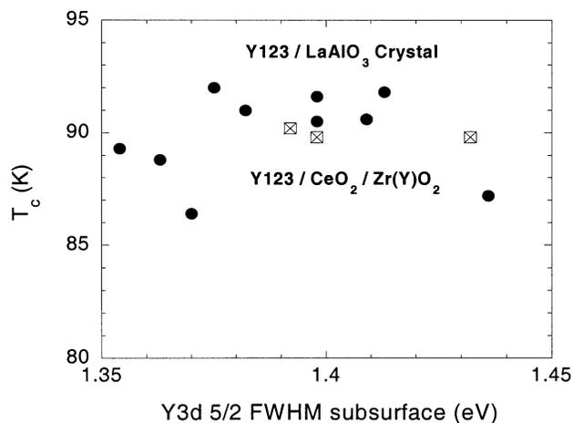
Fig. 3. The critical transition temperature of the samples as determined by magnetic susceptibility measurements are plotted versus the FWHM for the  $Y(3d_{5/2})$  peak as determined by XPS. No clear correlation is evident for the given data.
