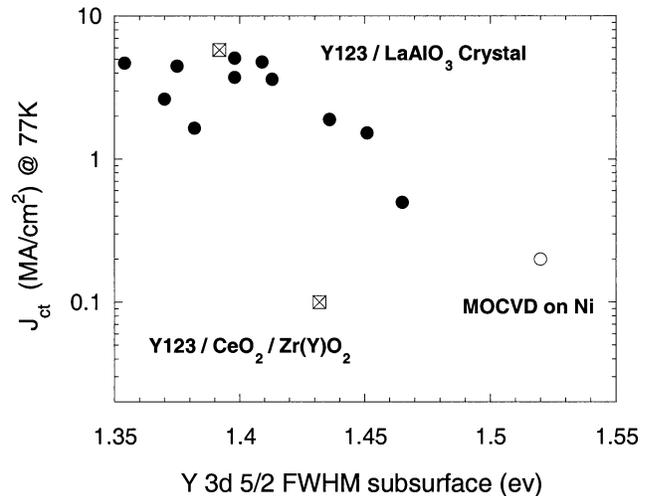
Fig. 1. Correlation of the FWHM for the  $\text{Y}(3d_{5/2})$  peak as determined by XPS and the critical transport current as determined by the four probe resistive technique. The sample preparation methods are labeled in the figure.
