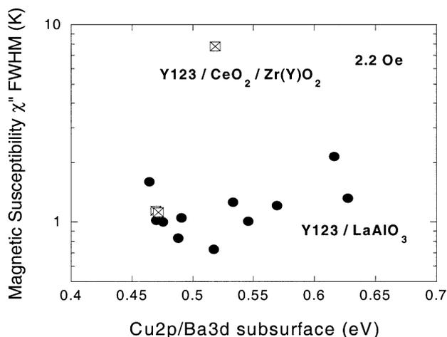
Fig. 5. Correlation of the peak intensity ratios for the  $Cu(2p)/Ba(3d)$  peaks as determined by XPS and the FWHM of the critical transition temperature as determined by magnetic susceptibility measurements.  $T_c$  data determined in 2.2 Oe magnetic field.
