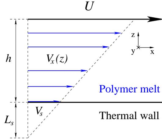
FIG. 1: (Color online) A schematic representation of the steady-state shear flow in the Couette cell. The upper wall is translated with a constant velocity  $U$  in the  $\hat{x}$  direction. The fluid slip velocity is determined from the relation  $V_s = \dot{\gamma}L_s$ , where  $\dot{\gamma}$  is the slope of the velocity profile and  $L_s$  is the slip length.
