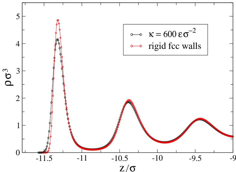
FIG. 1: (Color online) Averaged fluid density profiles near the thermal  $\kappa = 600 \varepsilon/\sigma^2$  ( $\circ$ ) and rigid ( $\diamond$ ) walls for  $\varepsilon_{\text{wf}}/\varepsilon = 0.9$  and  $f_x = 0.001 \varepsilon/\sigma$ . Left vertical axis coincides with the location of the liquid/solid interface at  $z = -11.79 \sigma$ .
