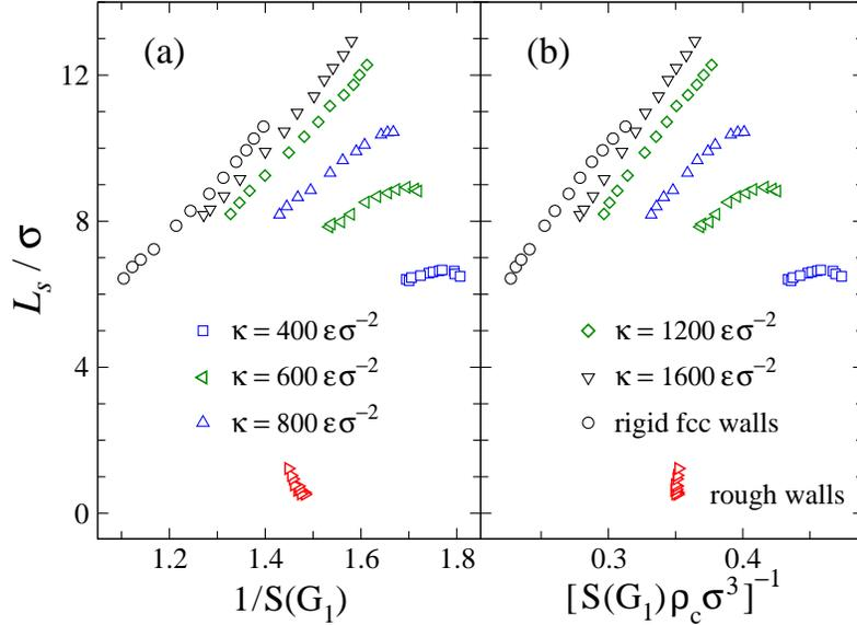
FIG. 4: (Color online) (a) Behavior of the slip length  $L_s/\sigma$  as a function of the inverse value of the in-plane structure factor,  $1/S(\mathbf{G}_1)$ , evaluated at the first reciprocal lattice vector  $\mathbf{G}_1 = (9.04 \sigma^{-1}, 0)$ . The wall-fluid interaction energy is  $\varepsilon_{\text{wf}}/\varepsilon = 0.9$ . (b) The same data for the indicated values of the spring constant are replotted versus  $[S(\mathbf{G}_1) \rho_c \sigma^3]^{-1}$ .
