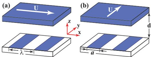
FIG. 1: (Color online) (a) Transverse and (b) longitudinal flow orientations for a liquid film subject to planar shear in a cell with wall separation  $d$ . Darker stripes of width  $a$  signify regions of finite slip or no-slip. White stripes signify regions of no-shear (or equivalently perfect slip). The upper wall moves at constant speed  $U$  relative to the lower stationary surface ( $z=0$ ). The periodicity of the lower wall pattern geometry is designed by  $\lambda$ .
