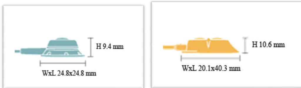
Figure 5 Sample port dimensions corresponding to the low profile titanium and the Rosenblatt models
