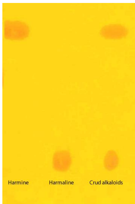
Figure 1: TLC for standards harmaline, harmine, and crud alkaloids detection with Dragendorff reagent.
