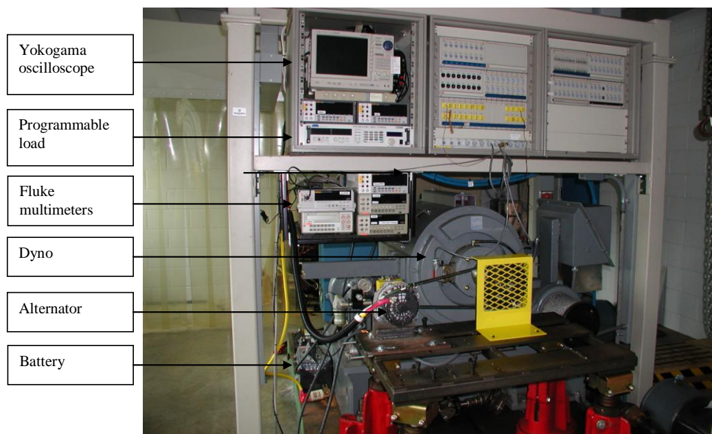
Figure 6: EPGS system test bench.
