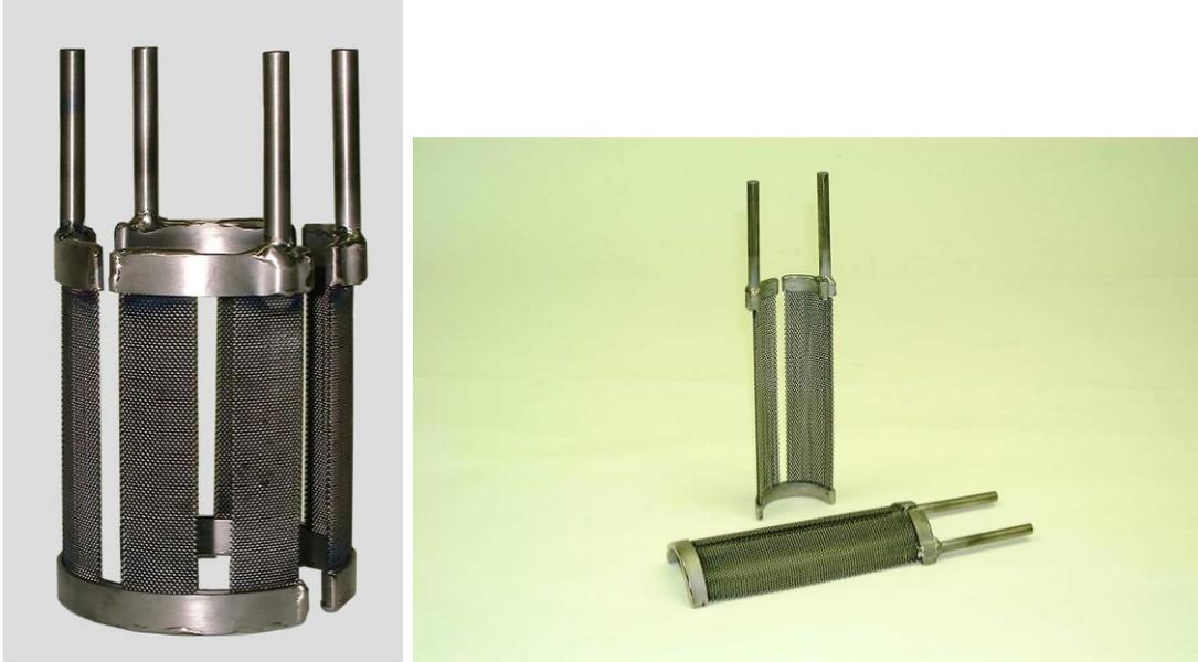
Figure 34. Tungsten heating elements.
