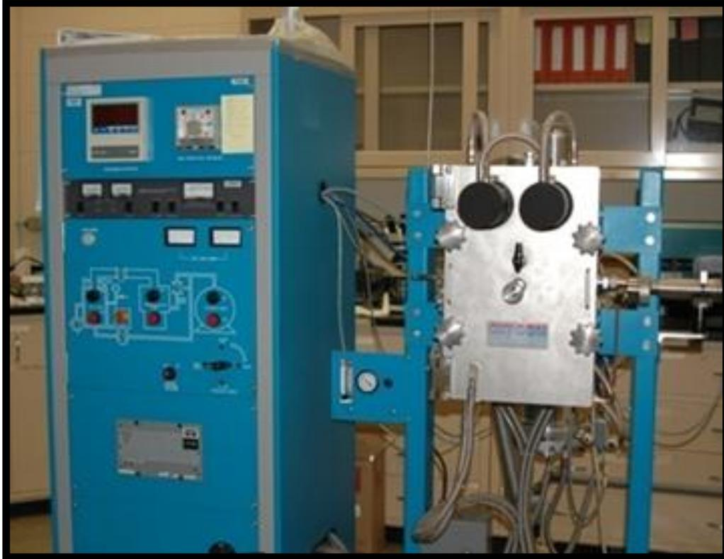
Figure 33. OxyGon furnace at AFRL.
