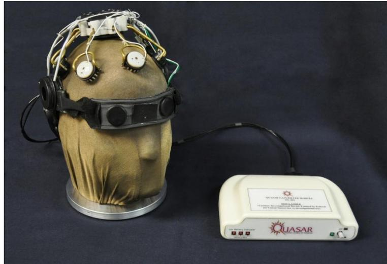
Fig. 1 Prototype dry electrode headset with wired amplifier/filter module.
