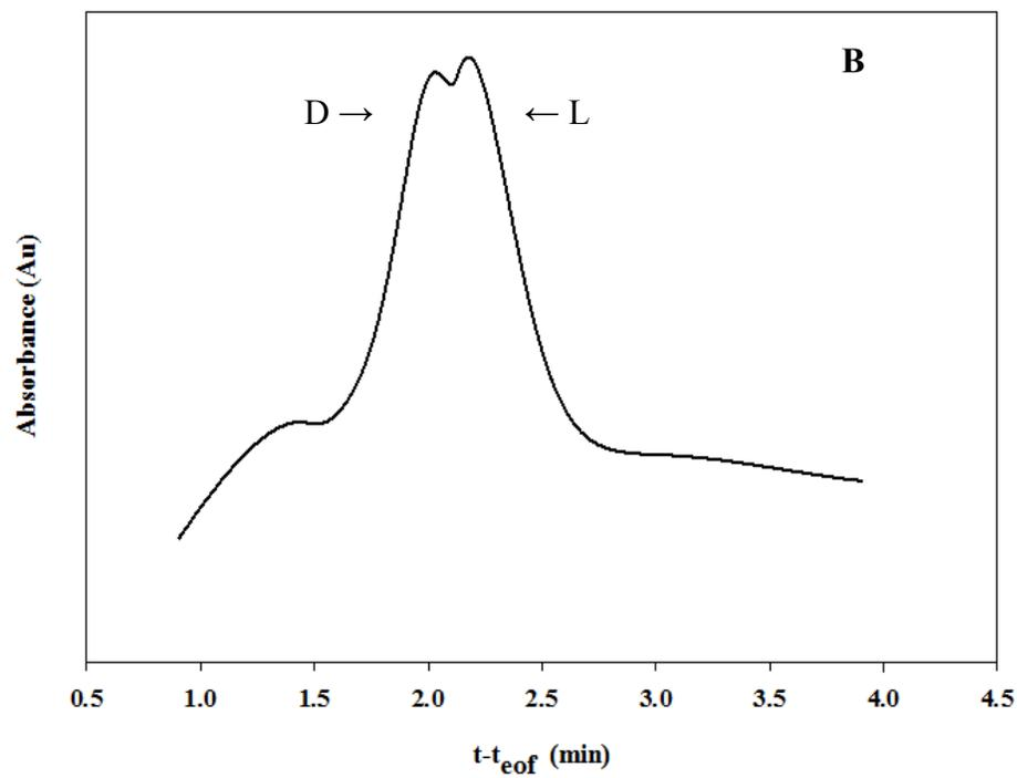
**Figure 45:** 5-fluoro-D,L-tryptophan (0.22 mg/ml) binding by unmodified BSA (A) and 1 week modified BSA (B). The serum protein concentration was held at 35  $\mu$ M. ACE conditions: 15 kV, 25°C, injection at 20 mbar for 5 s, and detection at 280 nm.
