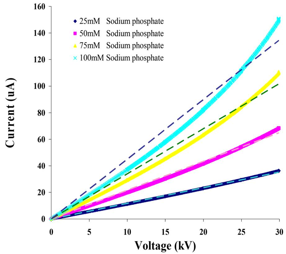
Although capillaries are cooled on the outer surface, a significant temperature difference between the BGE in the center and the inner capillary wall can occur leading to nonuniform temperature gradients within the capillary as well as localized changes in BGE viscosity. The generation of heat can evaporate BGE solution. Therefore heat dissipation should be efficient to avoid these adverse effects. Thermal effects can be circumvented by adjusting the ionic strength of the BGE.
