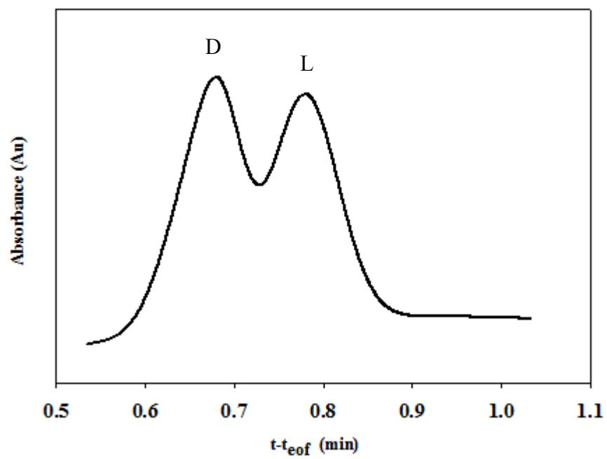
**Figure 39:** Electropharogram of 5-fluoro-D,L-tryptophan at a ibuprofen:BSA molar ratio of 1.6:1 (22  $\mu$ M ibuprofen). The serum protein concentration was held at 35  $\mu$ M. ACE conditions: 15 kV, 25°C, injection at 20 mbar for 5 s, and detection at 280 nm.
