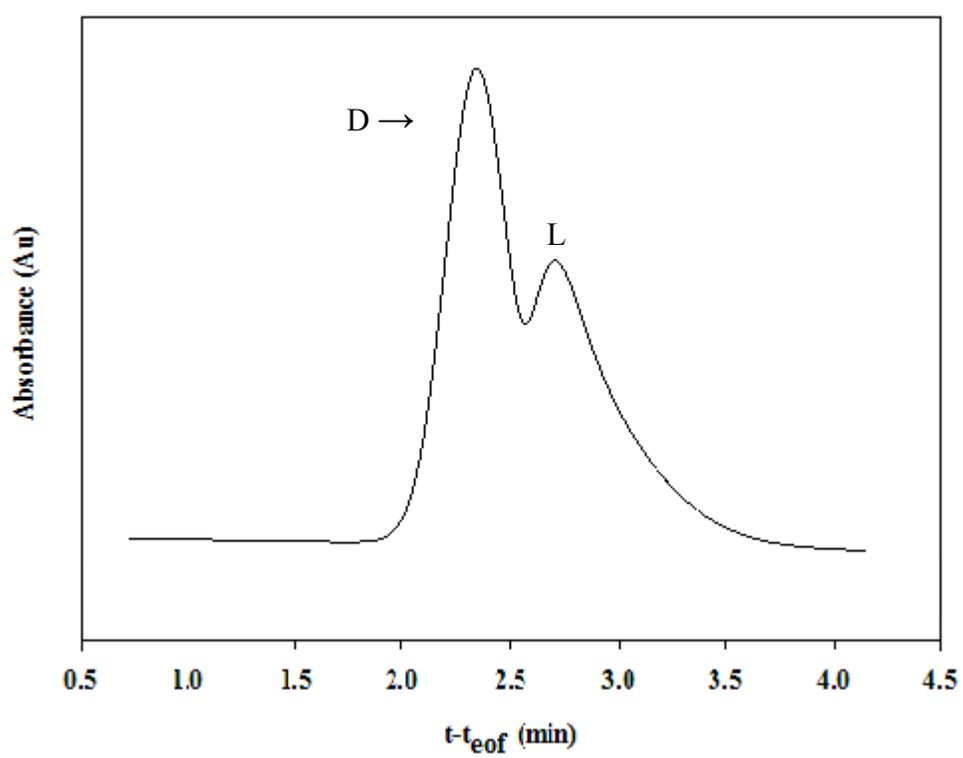
**Figure 30:** D,L-tryptophan (0.54mg/ml) prepared in 25 mM sodium phosphate, pH 7.4. ACE conditions: 25 mM sodium phosphate, pH 7.4, 30  $\mu$ M BSA, 25°C, 20 mbar injection for 5s, 15 kV, detection at 280 nm.
