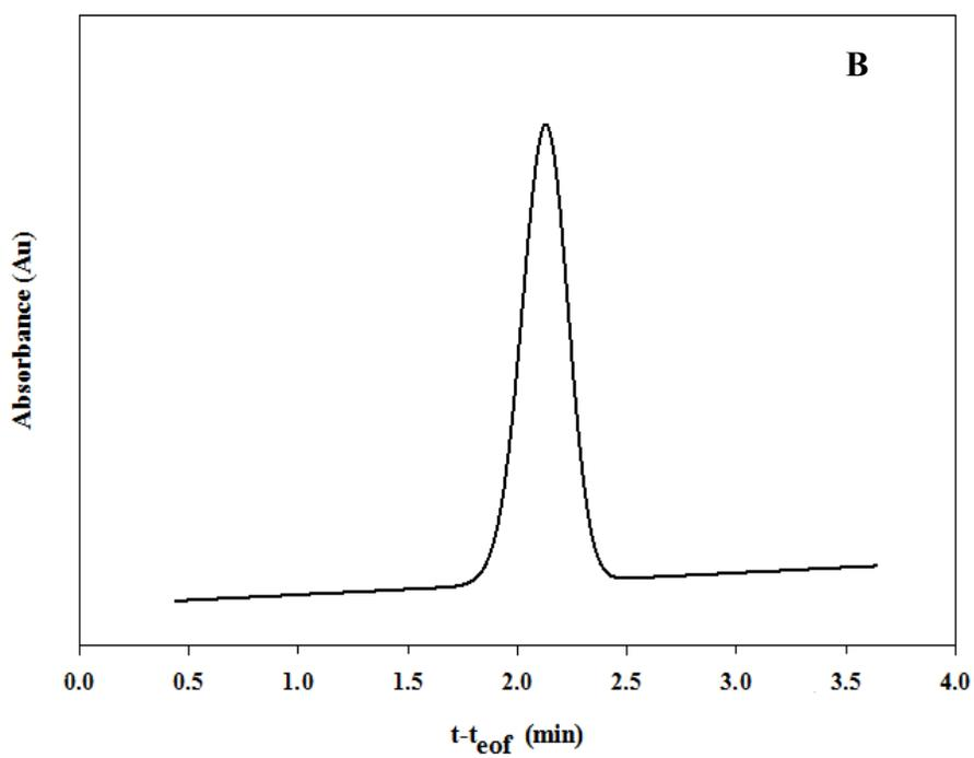
**Figure 48:** 5-hydroxy-D,L-tryptophan (0.22 mg/ml) binding by 2 week modified BSA (A) and 3 week modified BSA (B). The serum protein concentration was held at 35  $\mu$ M. ACE conditions: 15 kV, 25°C, injection at 20 mbar for 5 s, and detection at 280 nm.
