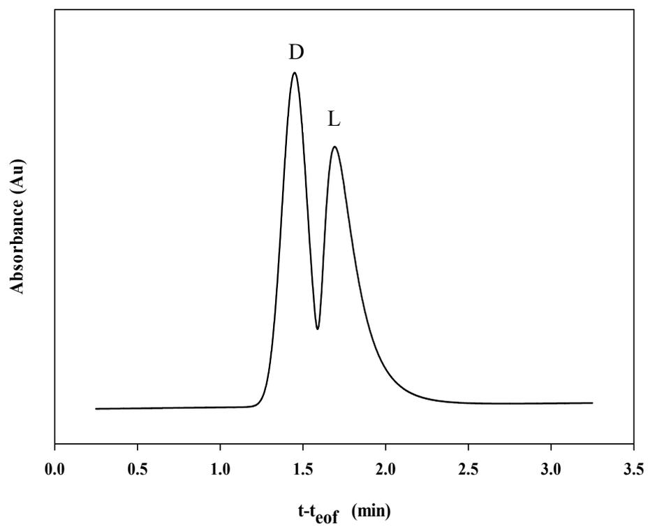
**Figure 24:** 60 minute wait. D,L- tryptophan (0.54 mg/ml). ACE conditions: 25 mM sodium phosphate, pH 7.4, 30  $\mu$ M BSA, 25°C, 20 mbar injection for 5s, 15 kV, detection at 280 nm. The capillary was rinsed for 8 minutes with background electrolyte solution prior to wait period.
