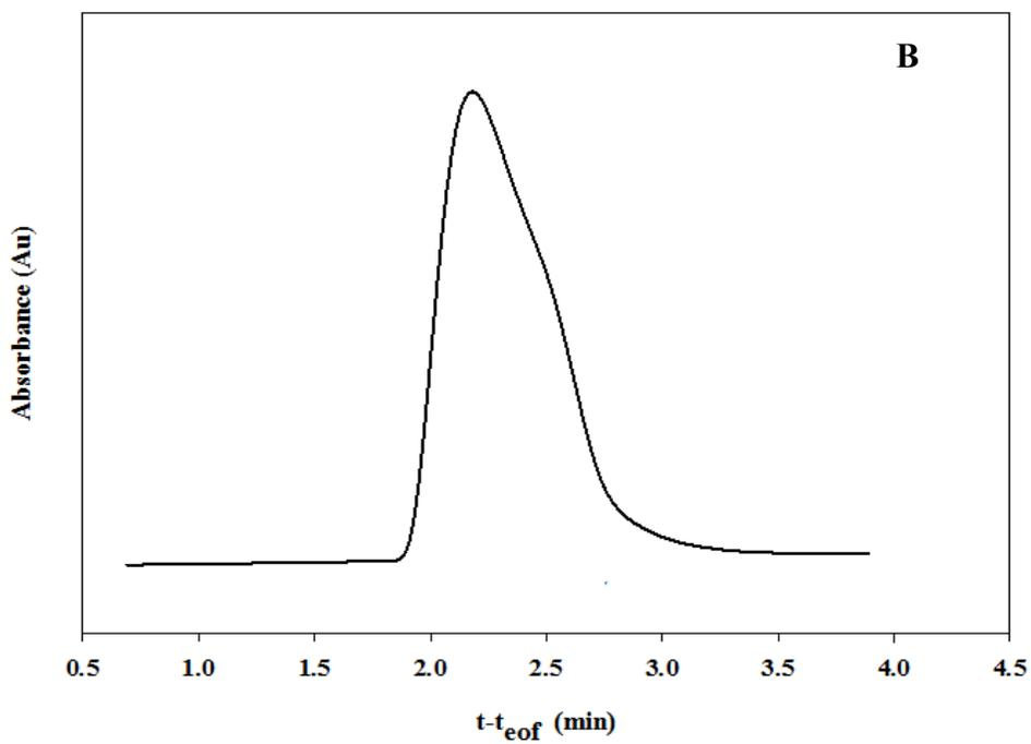
**Figure 44:** D,L-tryptophan (0.22 mg/ml) binding by 2 week modified BSA (A) and 3 week modified BSA (B). The serum protein concentration was held at 35  $\mu$ M. ACE conditions: 15 kV, 25°C, injection at 20 mbar for 5 s, and detection at 280 nm.
