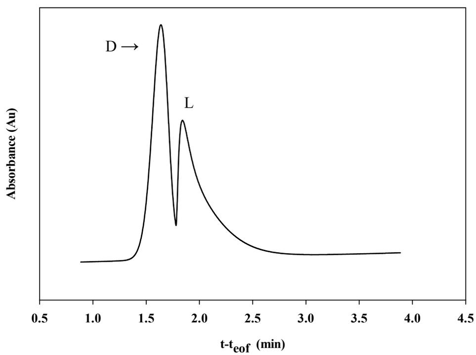
**Figure 28:** D,L-tryptophan (0.54mg/ml) prepared in 8 mM sodium phosphate, pH 7.4. ACE conditions: 25 mM sodium phosphate, pH 7.4, 30  $\mu$ M BSA, 25°C, 20 mbar injection for 5s, 15 kV, detection at 280 nm.
