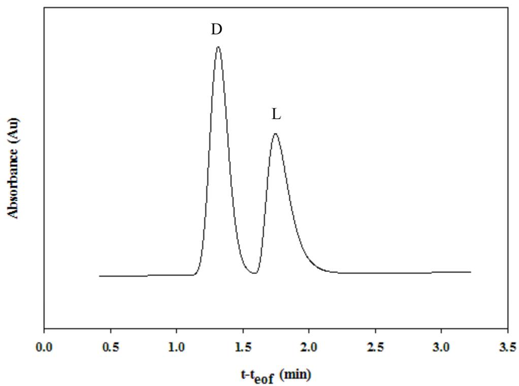
**Figure 23:** 40 minute wait. D,L-tryptophan (0.54 mg/ml). ACE conditions: 25 mM sodium phosphate, pH 7.4, 30  $\mu$ M BSA, 25°C, 20 mbar injection for 5s, 15 kV, detection at 280 nm. The capillary was rinsed for 8 minutes with background electrolyte solution prior to wait period.
