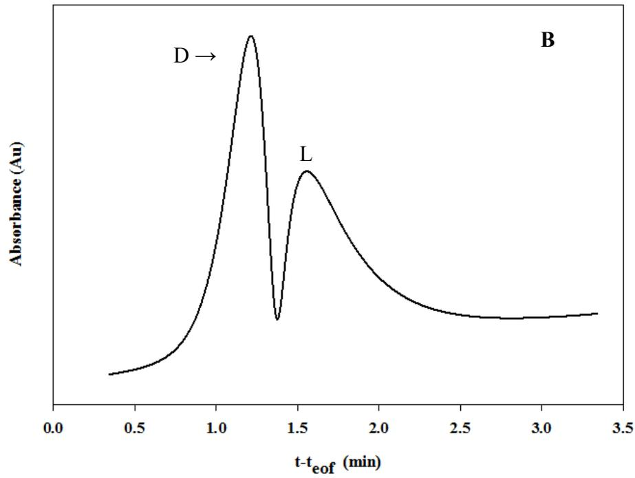
**Figure 46:** 5-fluoro-D,L-tryptophan (0.22 mg/ml) binding by 2 week modified BSA (A) and 3 week modified BSA (B). The serum protein concentration was held at 35  $\mu$ M. ACE conditions: 15 kV, 25°C, injection at 20 mbar for 5 s, and detection at 280 nm.
