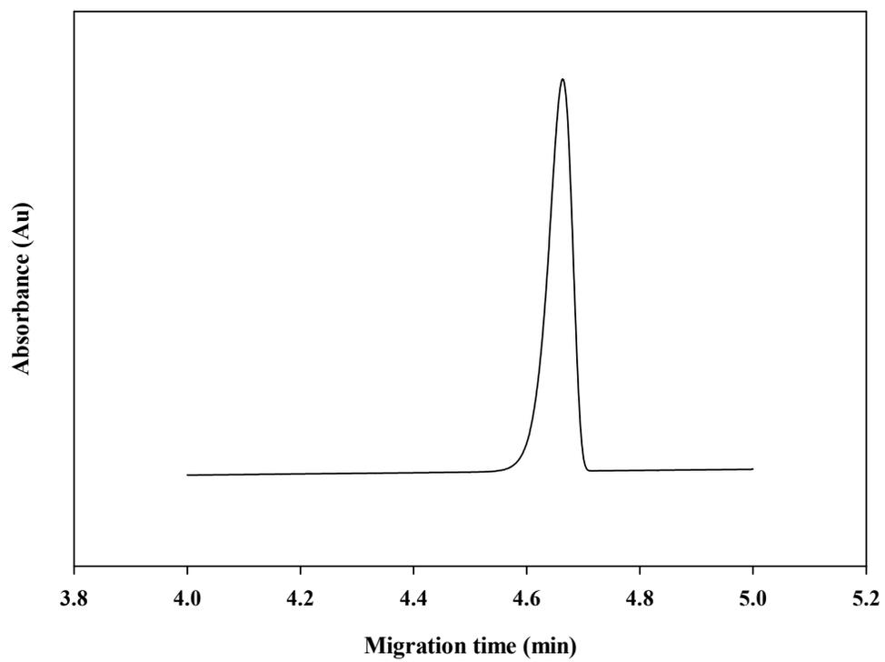
**Figure 36:** Changes in peak shape due to nonlinear isotherm conditions. BSA concentration was held to 35  $\mu$ M. D,L-tryptophan sample concentrations used were 0.1 mg/ml, 0.4 mg/ml, and 0.9 mg/ml. ACE conditions: 15 kV, 25°C, injection at 20 mbar for 5 s, and detection at 280 nm.
