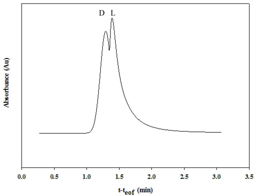
**Figure 17:** Electropherogram of D, L- tryptophan (0.54mg/ml) after rinsing the capillary for 24 min with BGE prior to applying the voltage. ACE conditions: 25 mM sodium phosphate, pH 7.4, 30  $\mu$ M BSA, 25°C, 20 mbar injection for 5s, 15 kV, detection at 280 nm.
