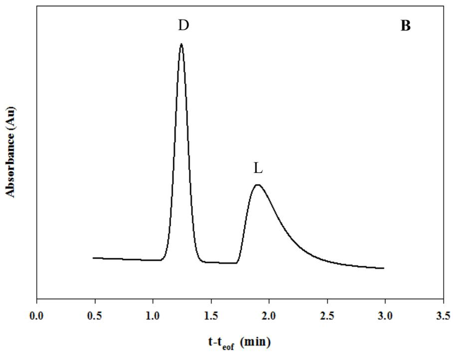
**Figure 47:** 5-hydroxy-D,L-tryptophan (0.22 mg/ml) binding by unmodified BSA (A) and 1 week modified BSA (B). The serum protein concentration was held at 35  $\mu$ M. ACE conditions: 15 kV, 25°C, injection at 20 mbar for 5 s, and detection at 280 nm.
