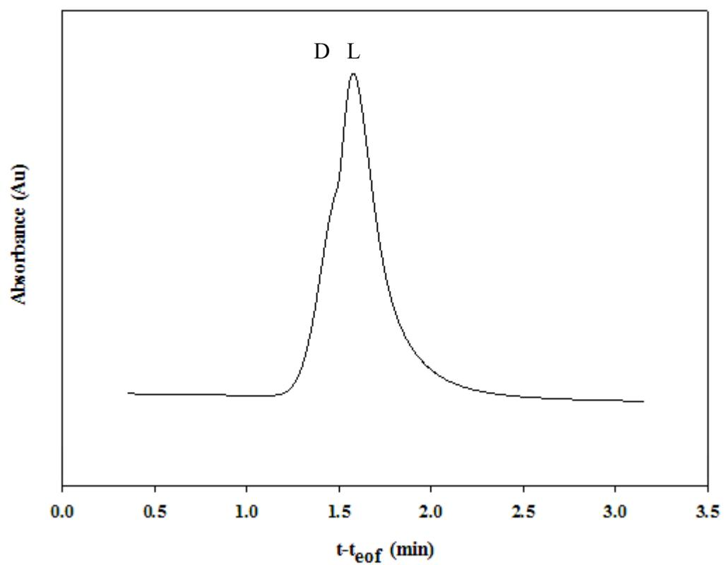
**Figure 18:** Electropharogram of D, L- tryptophan (0.54mg/ml) after rinsing the capillary for 32 min with BGE prior to applying the voltage. ACE conditions: 25 mM sodium phosphate, pH 7.4, 30  $\mu$ M BSA, 25°C, 20 mbar injection for 5s, 15 kV, detection at 280 nm.
