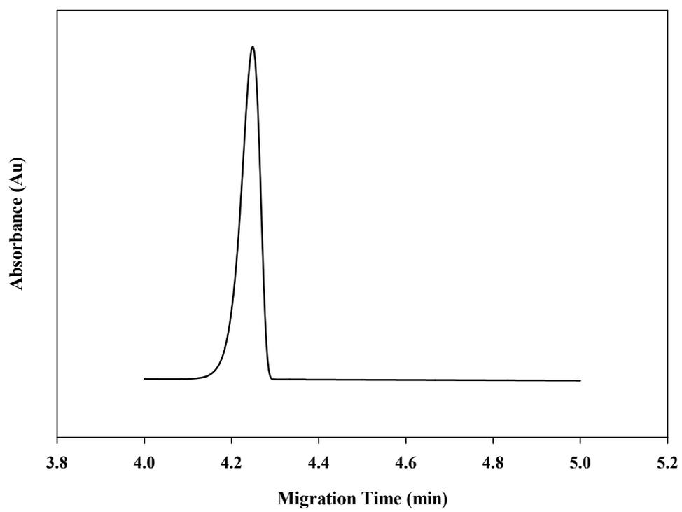
**Figure 35:** 5-fluoro-D,L-tryptophan, 0.22 mg/ml (1mM), run in 25 mM sodium phosphate, pH 7.4, void of BSA. ACE conditions: 15 kV, 25°C, injection at 20 mbar for 5 s, and detection at 280 nm.
