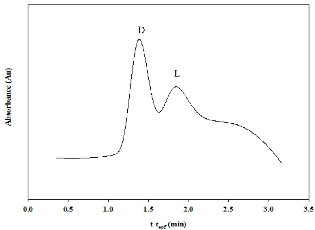
**Figure 12:** Effect of applied voltage on D- and L-tryptophan separation as represented by peak distortion. BSA concentration in BGE was kept at 30  $\mu\text{M}$  and D,L-tryptophan amount used was 0.54 mg/ml. ACE conditions: 25°C, 20 mbar injection for 5s, detection at 280 nm, 15 kV separation voltage.
