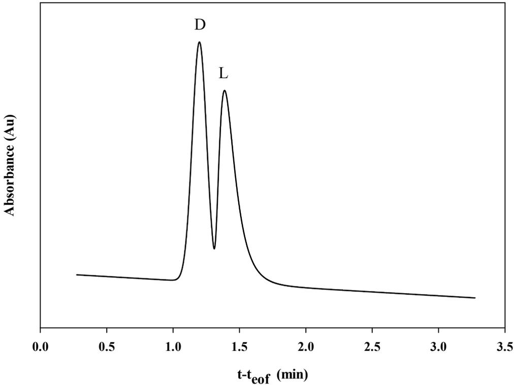
**Figure 16:** Electropherogram of D, L- tryptophan (0.54 mg/ml) separation after rinsing the capillary for 16 min with BGE prior to applying the voltage. ACE conditions: 25 mM sodium phosphate, pH 7.4, 30  $\mu$ M BSA, 25°C, 20 mbar injection for 5s, 15 kV, detection at 280 nm.
