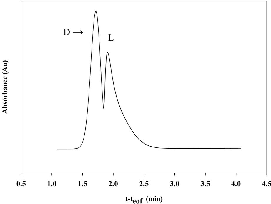
**Figure 29:** D, L-tryptophan (0.54mg/ml) prepared in 15 mM sodium phosphate, pH 7.4. ACE conditions: 25 mM sodium phosphate, pH 7.4, 30  $\mu$ M BSA, 25°C, 20 mbar injection for 5s, 15 kV, detection at 280 nm.
