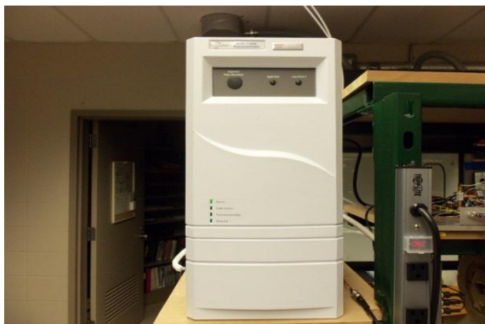
Figure 19 : The Entech 7100A Preconcentrator
