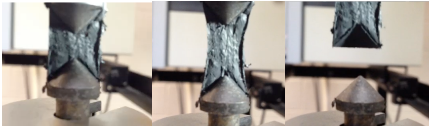
Figure 64: SPC before pull (left), during pull (center), and after pull (right).
