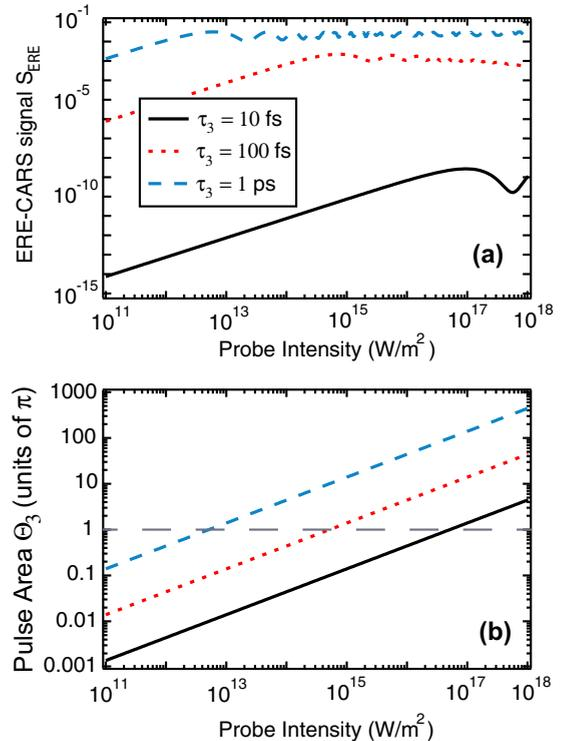
FIG. 3. Saturation of ERE-CARS signal intensity for different pulse durations in the hybrid ERE-CARS configuration. Pump- and Stokes-pulse durations are maintained at  $\tau_1 = \tau_2 = 100$  fs and only the probe-pulse duration  $\tau_3$  is varied. (a) The ERE-CARS signal  $S_{\text{ERE}}$  plotted as a function of peak intensity of the probe  $I_{30}$  and (b) pulse area  $\Theta_3$  corresponding to  $I_{30}$ .
