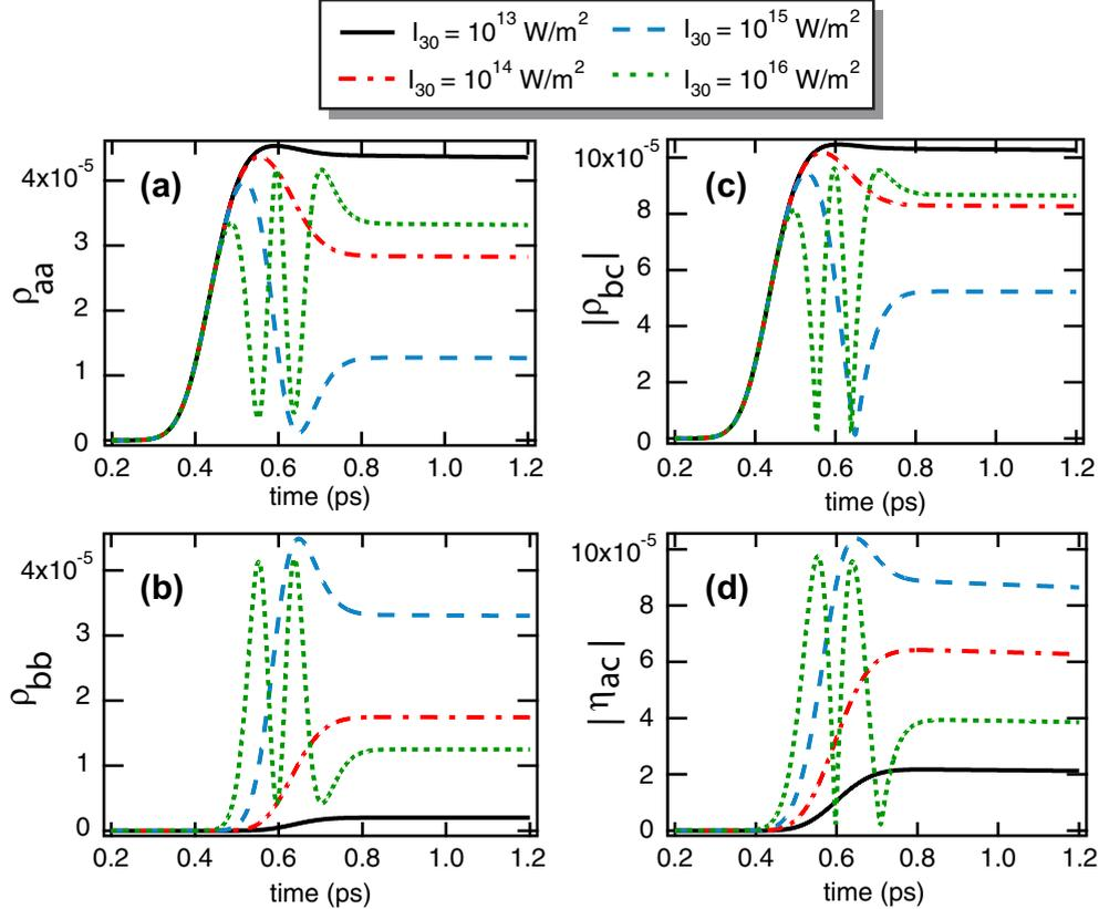
FIG. 2. (a) Population in the excited electronic state  $|a\rangle$ , (b) excited vibrational state  $|b\rangle$ , (c) ground-state (Raman) coherence, and (d) instantaneous polarization in the ERE-CARS transition for different probe intensities. The following parameters are used for the plot: the peak of the pump and Stokes pulse appears at 400 fs and the probe delay is maintained at 200 fs.
