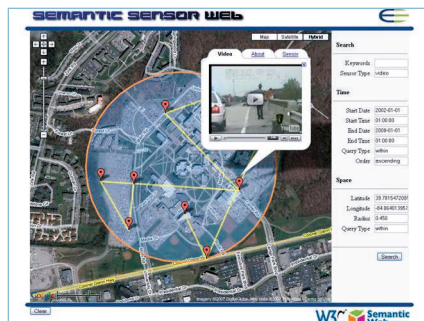
Figure 3. A semantic mashup with ability to show videos that capture events from police cruiser cameras with user queries on spatial region and time interval.
