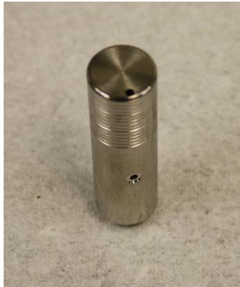
Fig. 8: Atomizer within the Optomec AJDT system
