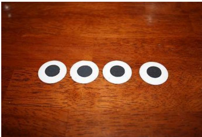
Fig. 9: A set of four completed fuel cells with the black LSCF layer visible on top
