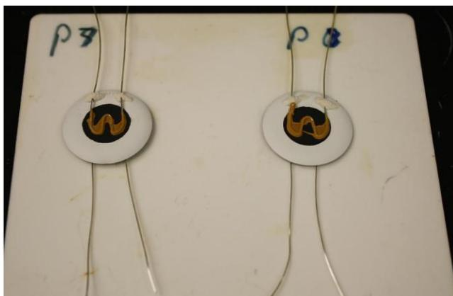
Fig. 10: Fuel cells with silver wire test leads in M-shape configuration
