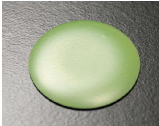
Fig. 5: Bisque-fired anode substrate
