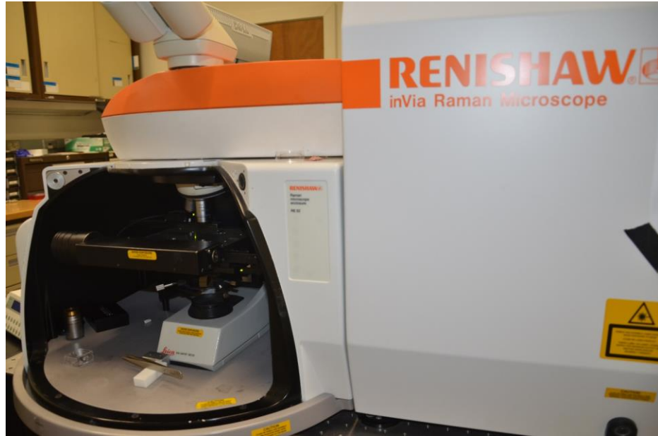
Figure 6.1. Raman spectrometer. Samples analyzed for graphene-based peaks.
