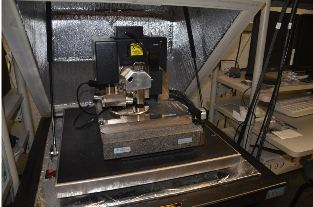
Figure 6.2. Atomic Force Microscopy system. In this research, the tapping mode was used on each sample.
