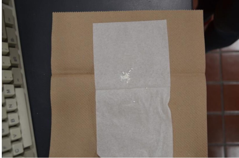
Figure 4.1. Guanine powder prior to physical vapor deposition onto substrates.
