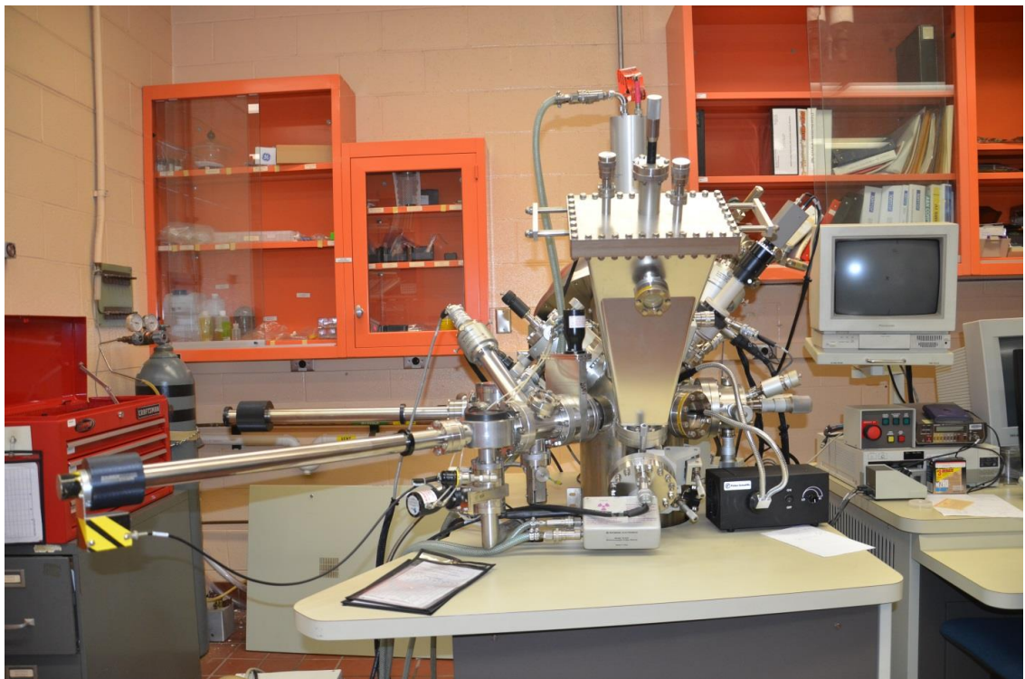
Figure 6.6. X-ray photoelectron spectroscopy image of sample measurement setup. Graphene-based samples were analyzed for impurities.
