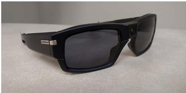
Fig. 1. Pivothead Glasses with Embedded Camera
