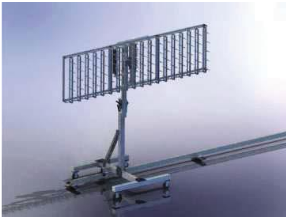
Figure 9. Planar Array Constructed for a NAH Measurement (James, et al., 2011)
