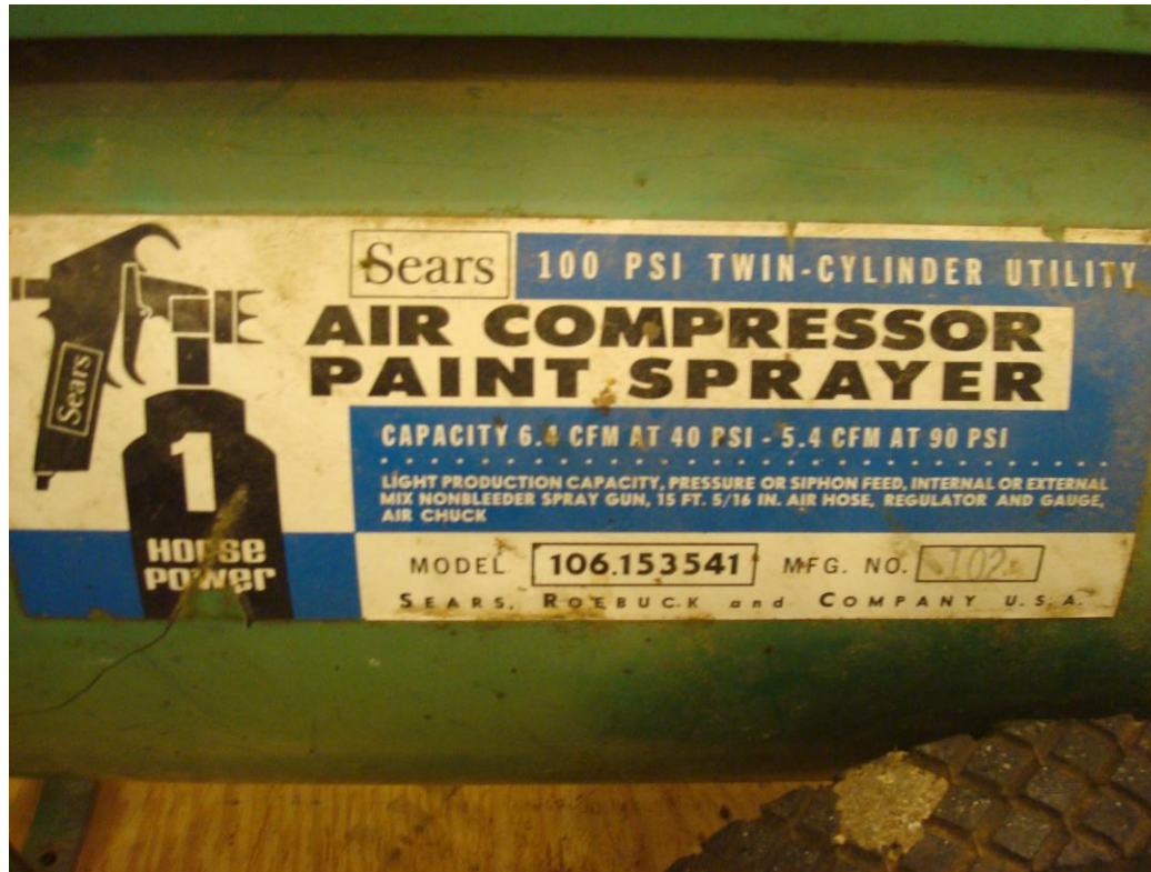
Figure 21. Air Compressor Model and Information Sticker
