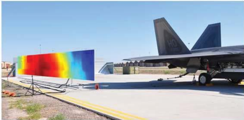
Figure 10. Measured SPL Map Overlaid on a F-22 Photo at the Approximate Location of Measurement (James, et al., 2011)
