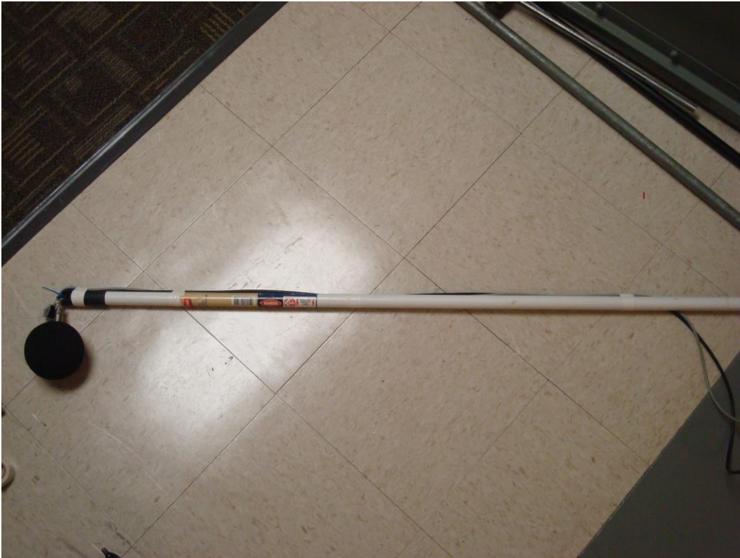
Figure 20. Assembled array with the G.R.A.S. microphone and the head-tracker sensor incorporated with a 5 foot dowel.
