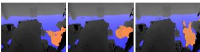
Figure 2. Hospital fall; blue area for ground and the orange object as foreground after using an adaptive background subtraction algorithm.
