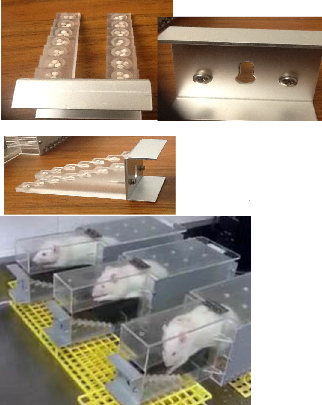
Figure 1: Montoya staircase apparatus
