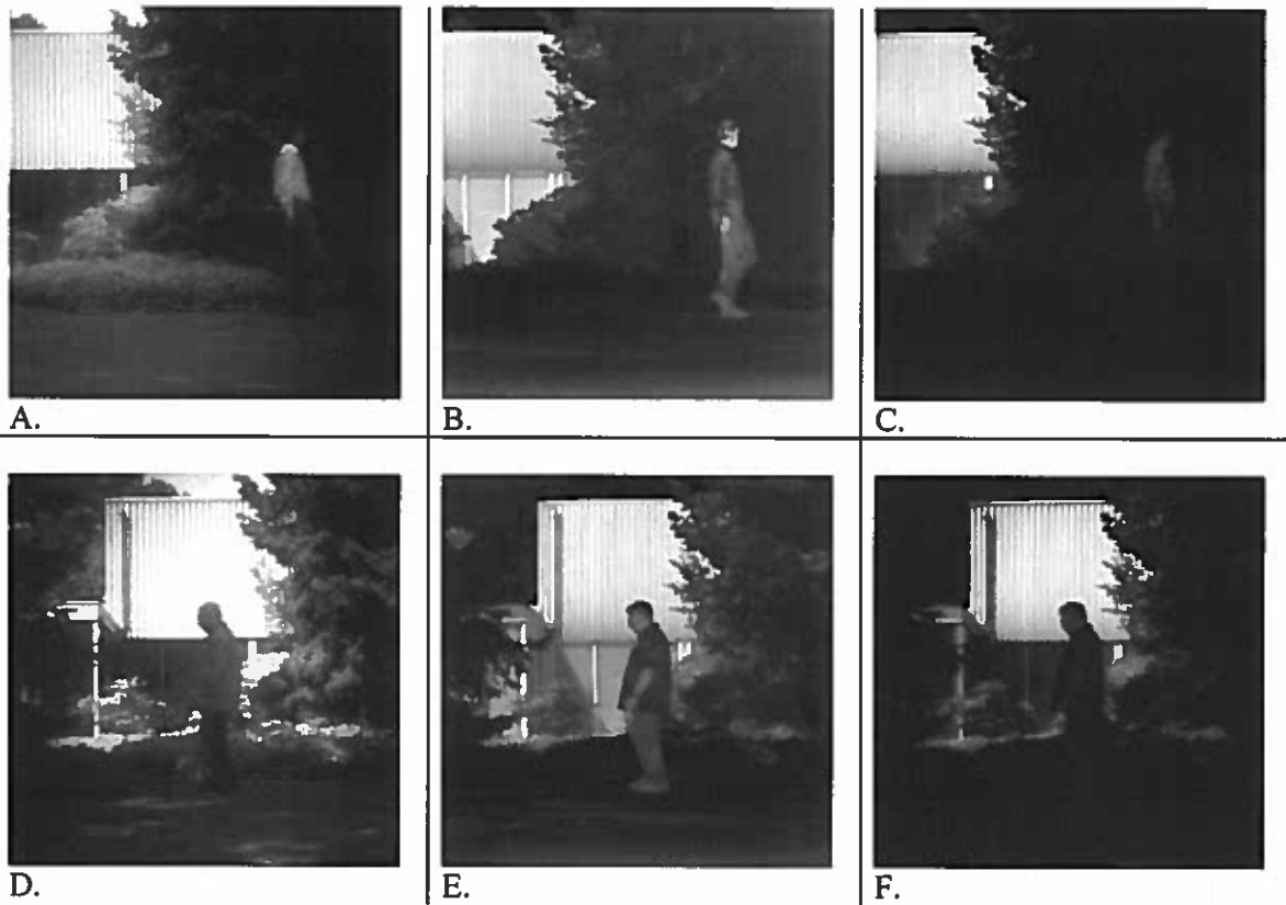
Figure 33. An example of each target either facing left in the visible-only (A), LWIR-only (B), and Laplacian algorithmically fused (C) image or facing right in the visible-only (D), LWIR-only (E), and Laplacian algorithmically fused (F) used in Experiment 2.
