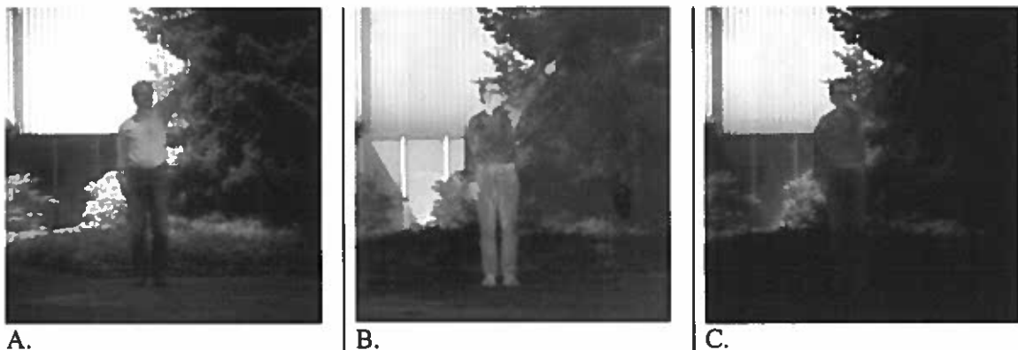
A. B. C. Figure 1. An example of a visible (A), long-wave infrared (B), and the combination of 1A and 1B using the Laplacian fusion algorithm (C). I used these images for the discrimination task in Experiment 1 (discussed in later sections).
