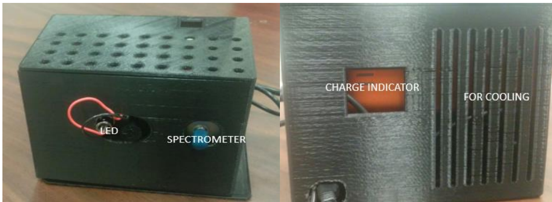
Figure 4.12: Front and side view of the spectrometer module
