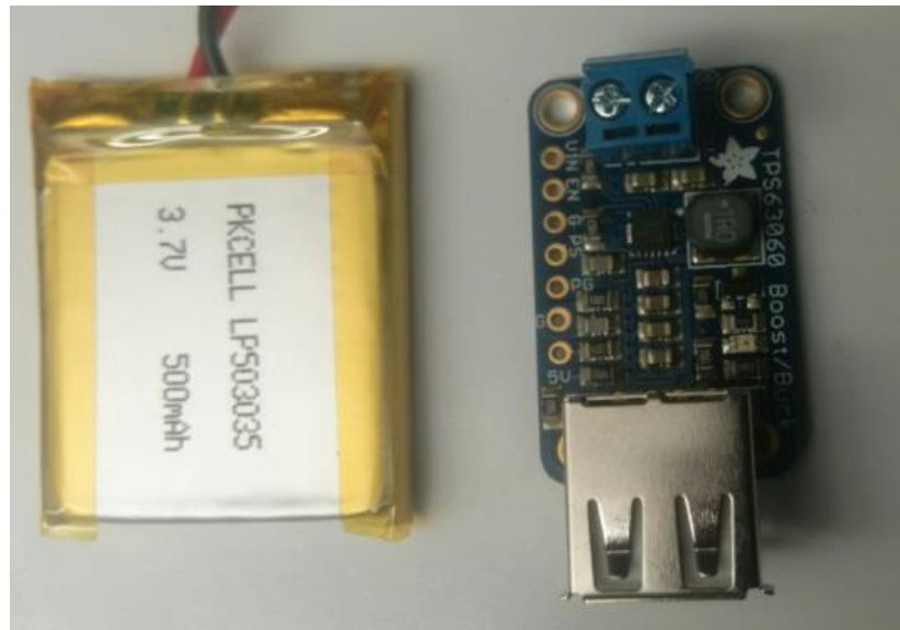
Figure 3.22: Battery and charger
