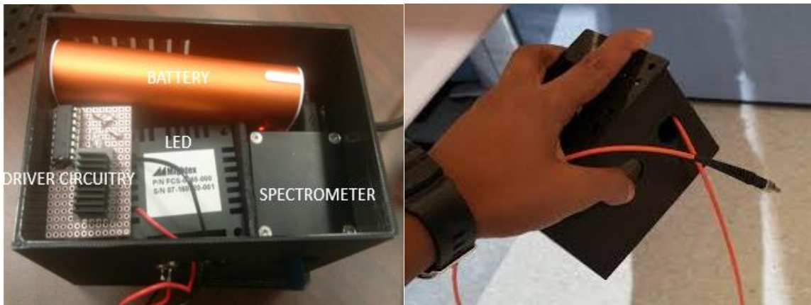
Figure 4.13: Top view of spectrometer module
