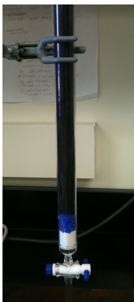
Figure 2.10. The column used to purify EMIBF 4 .
