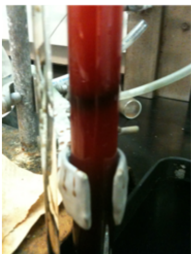
Figure 2.8 The Mo 3 trimer in the ion-exchange column with 1.0M trifluoromethanesulfonic acid added.
