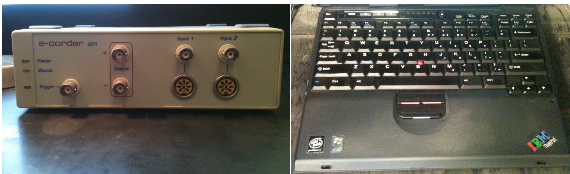
Figure 2.18. The model 201 eDAQ eCorder data capture device, used with an IBM ThinkPad laptop PC.
