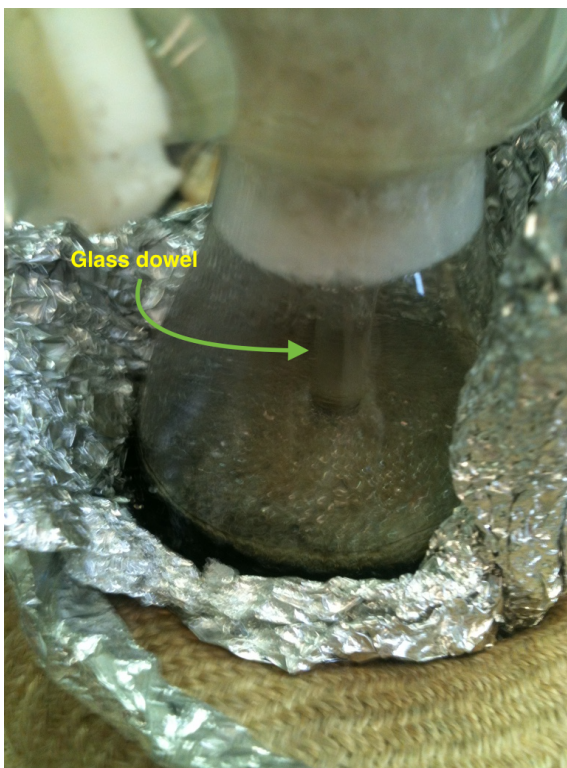
Figure 2.4 A glass dowel helps to keep the neck of the condenser free of obstruction.
