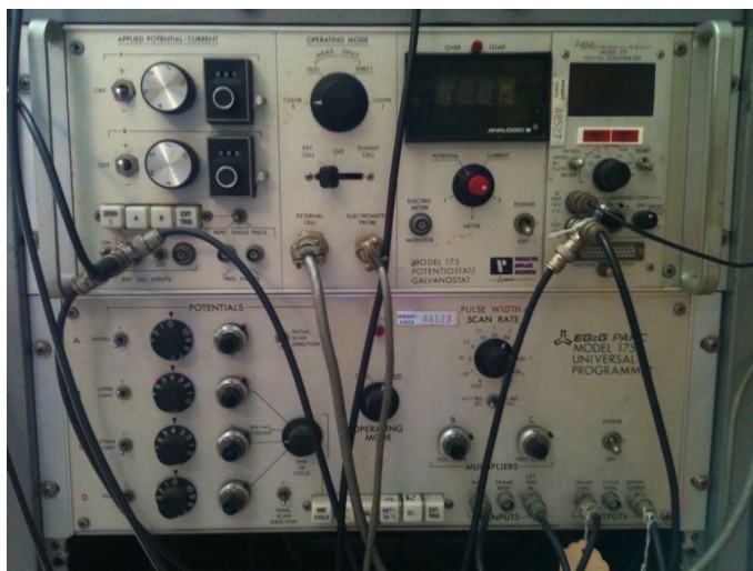
Figure 2.17. The Princeton Applied Research/EG&G model 173 Digital Potentiostat/Galvanostat equipped with model 179 Digital Coulometer linked to a model 175 Universal Programmer.
