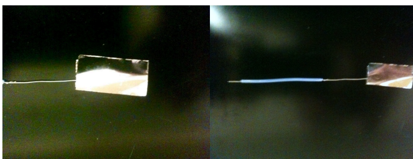
Figure 2.16. The bare Pt-foil electrode above is an example of the type of electrode used.
