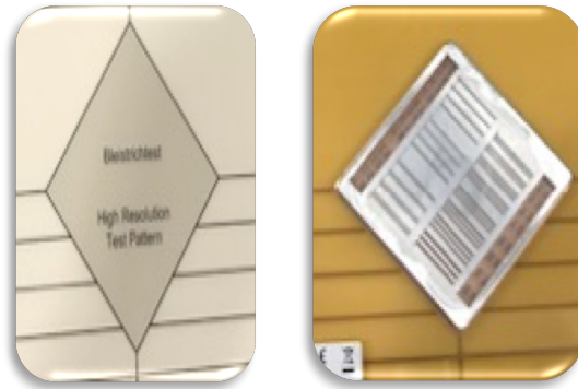
Figure 17 Test pattern that used to measure contrast (image from test object Normi 13 phantom)
