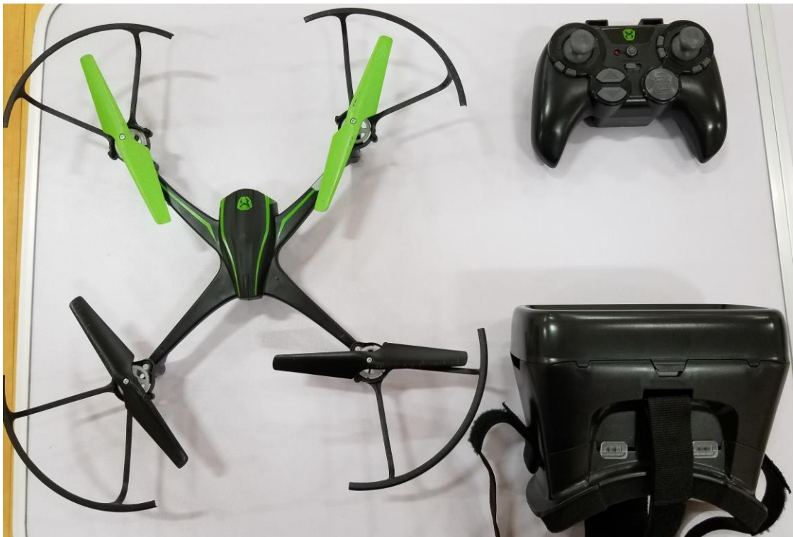
Figure 6: The SkyViper v2400fpv drone that is used in this study, as well as the controller and the FPV headset.
