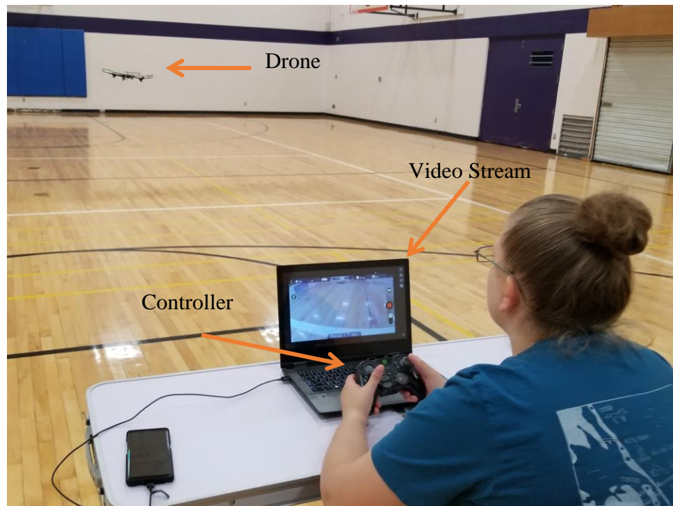
Figure 2: Video aided control interface method. The operator can see the video stream from the front mounted camera on the drone, as well as maintain visual line of sight.
