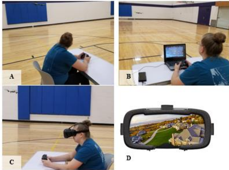
Figure 4: A) LOS control interface method. B) Video aided control interface method. C) FPV control interface method. D) A generic view for the operator while using FPV to operate the drone.
