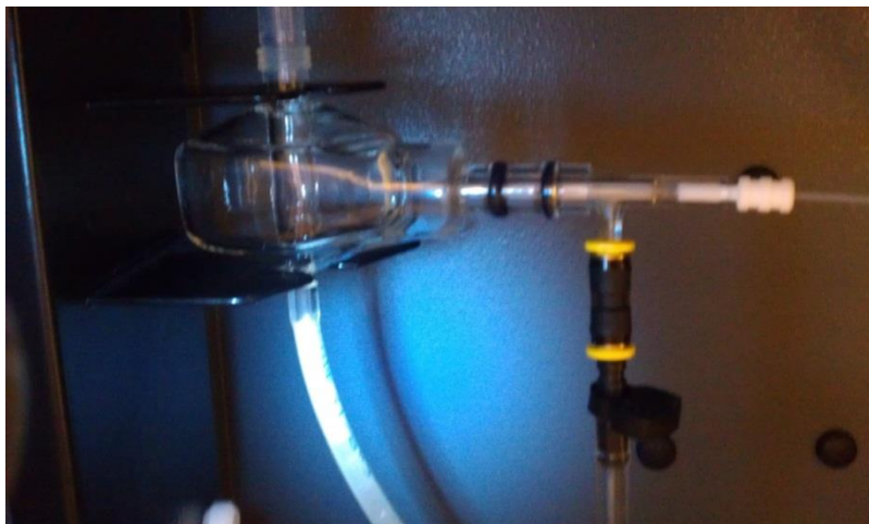
Figure 9: Photo of the ICP-OES nebulizer taken while the plasma was on. It illustrates its location at the right side of the spray chamber with respect to the operator (710 Varian/Agilent – Instrumental Analysis Lab).
