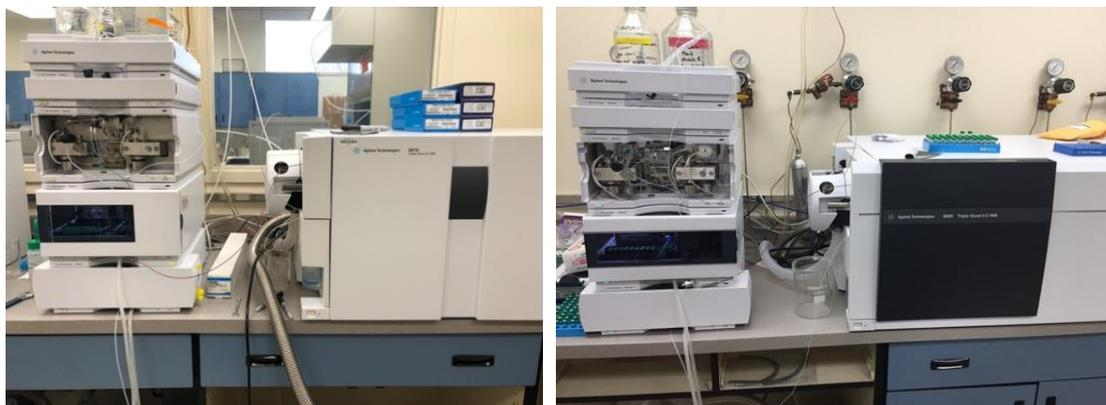
**Figure 2.** Left: Image of a 1200 series LC system coupled with a 6410 triple quadrupole. Right: Image of an HPLC 1260 Infinity system coupled to a 6420 triple quadrupole (reproduced with permission of the Montgomery County Coroner's Office laboratories).
