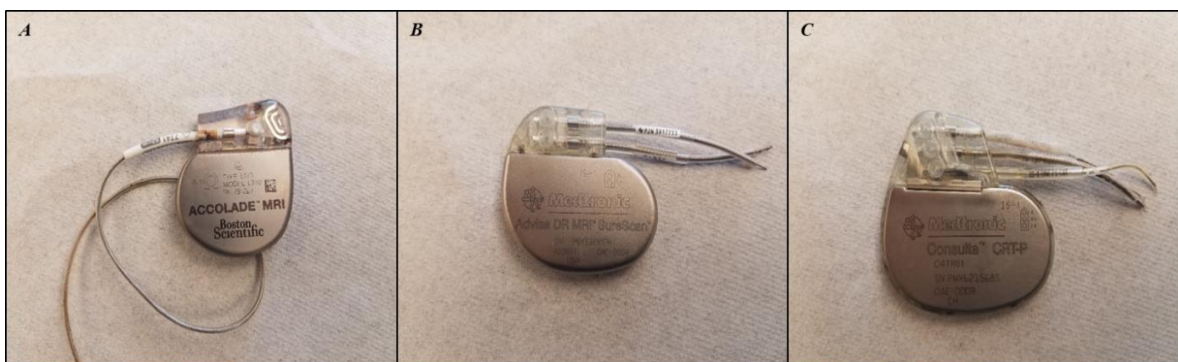
Figure 1 A) Single chamber pacemaker, B) Dual chamber pacemaker, C) Triple chamber pacemaker (CRT-P)
