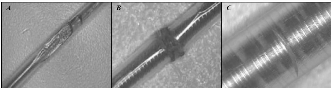
Figure 14 A) thermal damage on PU55D B) thermal damage on PU55D C) mechanical damage on silicone [55]
