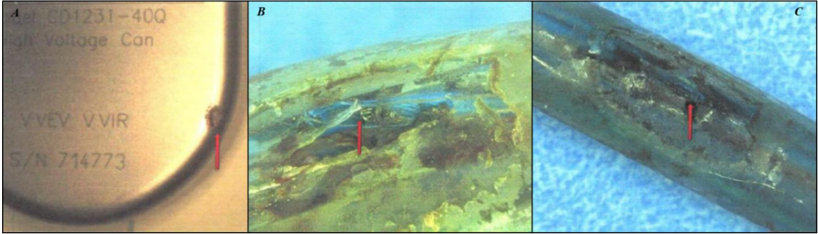
Figure 13 A) Pulse generator discoloration B) ETFE abrasion C) External abrasion [52]
