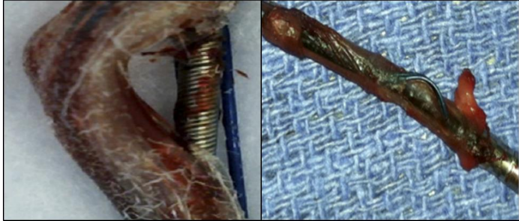
Figure 11 Showing insulation break due to fluoroscopy, and how the coil is damaged [51]
