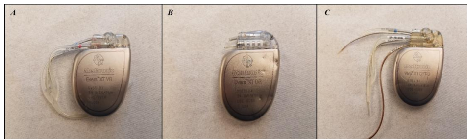
Figure 2 A) Single chamber ICD B) Dual chamber ICD C) Triple chamber ICD (CRT-D)
