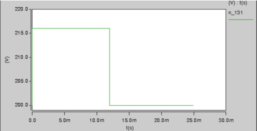
Figure. 5.2. Input Voltage with Step Change
