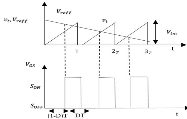
Figure 4.2. Feed-Forward Circuit Waveform
