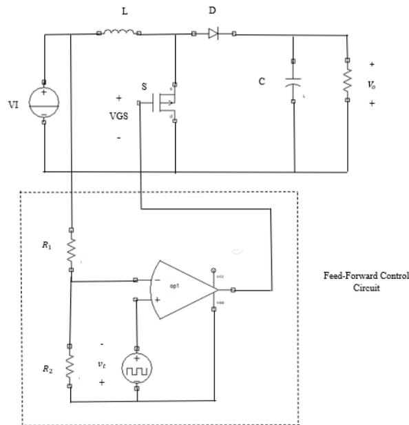
Figure. 3.4 Feed-Forward Circuit
