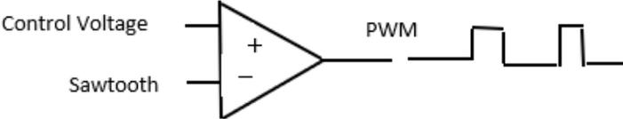
Figure. 3.5 Comparator Circuit
