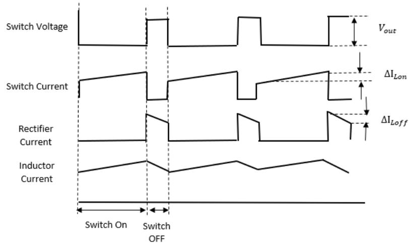
Figure. 3.3 CCM Waveform
