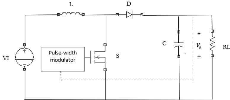
Figure. 3.1 Equivalent Circuit for the PWM Boost Converter
