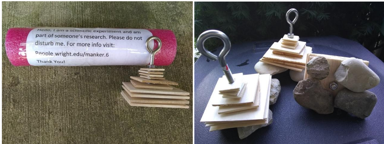
Figure 9. Photo of Hester-Dendy sampler. Hester-Dendy sampler constructed as per instructions listed in the methods section. Styrofoam buoy labeled as a research device and listing contact info for the curious (left). Modified Hester-Dendy (right).
