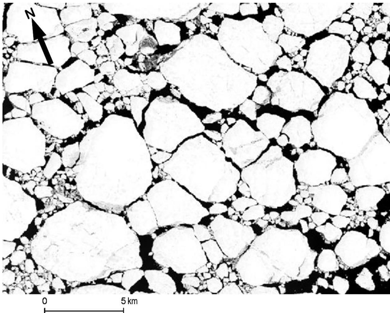
Figure 5b. (07 December 2015) Close up of satellite image soon after the initial breakup of sea ice by the process of fracture. The irregular lines visible within each floe are fused boundaries between old floe that compose the ice pack. See Figure 4a for location. Image Number LC08\_L1GT\_200106\_20151207 USGS Earth Explorer <https://earthexplorer.usgs.gov/>
