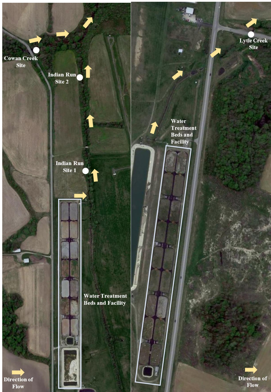
Figure 2 Satellite view of sample sites with direction of water flow, water treatment beds, and facilities displayed. [25]
