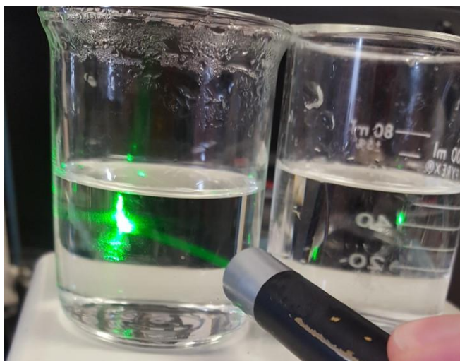
Figure S38 shows the laser pointer experiment for calcium fluoride ( [F^-] = 12.8 \text{ mM} ) where the laser is being pointed at the reaction cell.
