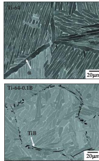
Fig. 5 — These backscattered electron images demonstrate how a trace boron addition reduces the thickness of the brittle grain boundary alpha phase.
