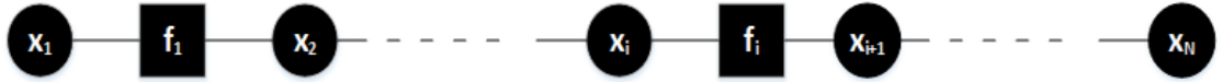
Figure 3.1: A Factor graph depiction of a Markov chain representing the random variability of a single endmember
